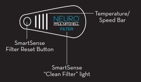
PRESS THE POWER BUTTON to turn on the hair dryer. The temperature/speed bar, logo, and "Clean Filter" will light up.
